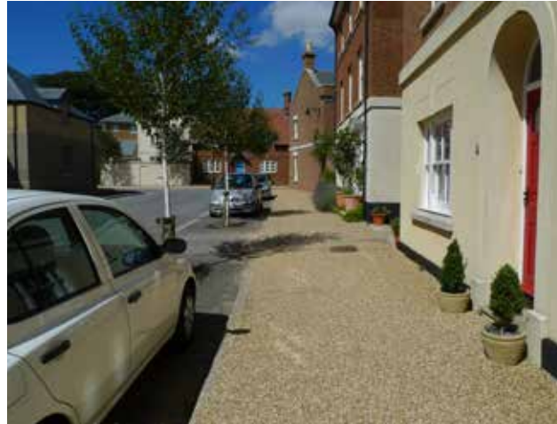
Figure 33: Example of on-street parking with parking bays and street trees to mitigate the impact of cars on the streetscape, Poundbury.
